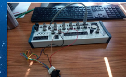
MPX5010DP Pressure sensor connected to BNC-2120
