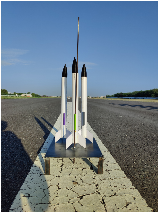
Figure: 58 These purple, green and grey tubes on rocket body are launch lugs
