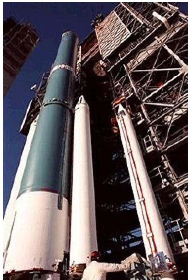
Figure 20: NASA Image of a solid rocket booster (right) being mated to a Delta II rocket (teal)
