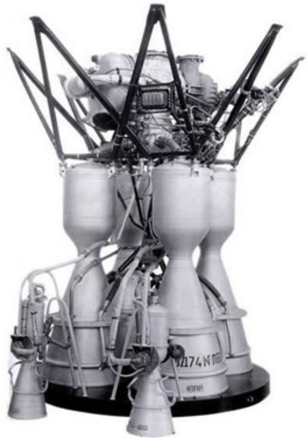
Figure 26: RD-107 gas-generator engine powers Russia's famous Soyuz rockets (NPO Energomash)
