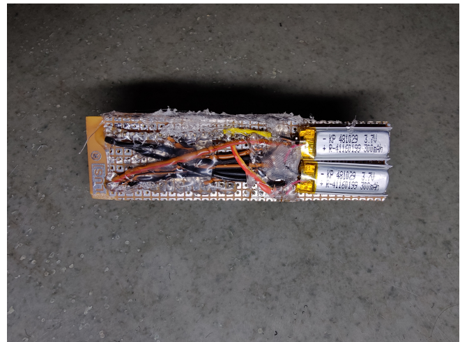
Figure: 63 Power source for altimeter and accelerometer
