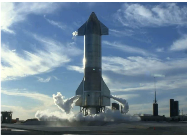
Figure 28: Starship fitted with SpaceX's powerful full-flow staged combustion Raptor Engines (SpaceX)
