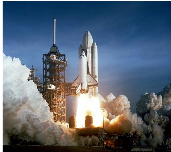
Figure 16: The Space Shuttle used both solid and liquid propellants.
